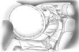
The front outboard passenger frontal airbag is in the passenger side instrument panel.
