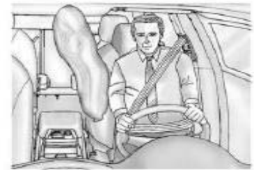
If the vehicle has a front center airbag, it is in the inboard side of the driver seatback.
