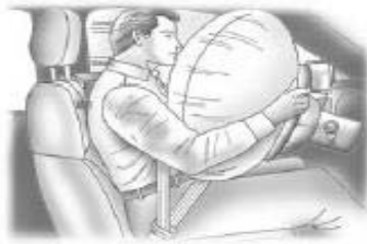
The driver frontal airbag is in the center of the steering wheel.
