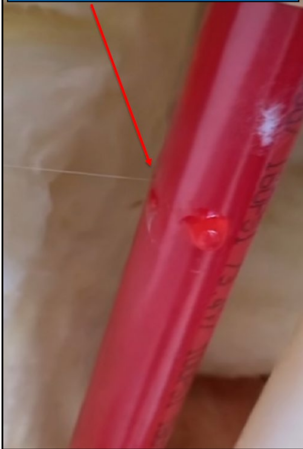
Image 6 – Cracked and leaking Uponor PEX red pipe away from fitting
